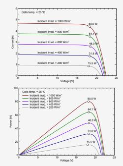
STC: Irradiance 1000W/m<sup>2</sup>,Module temperature 25°C, AM1.5 spectrum.
